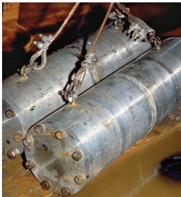
Fig. 78. Lycopodium Apparatus (LydiA) for injecting solid tracers into flooded underground mines. Diameter 120 mm.
